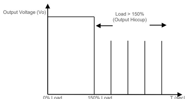
Additionally, if the  $I_o$  is  $< 210\%$  but  $> 150\%$  for a prolonged period of time (depending on the load), the Over Temperature Protection (OTP) will be activated due to high temperature on critical components. The power supply will then go into hiccup mode until the fault is removed; and, the input voltage is removed, then reapplied.
